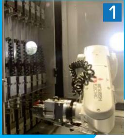
The first robotic arm is used for automatic loading of objects.
